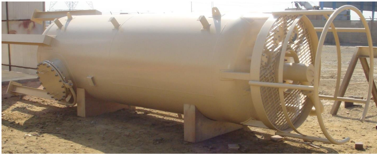
10 CU.MTR. SURGE VESSEL
