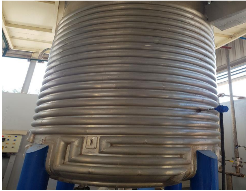
SS316L SS REACTOR WITH LYMPED COILS
