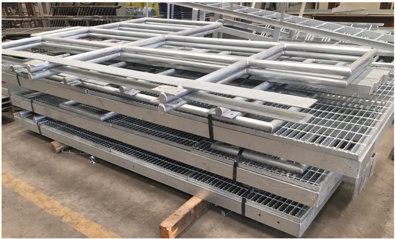
GALVANISED PLATFORMS AND HANDRAILS
